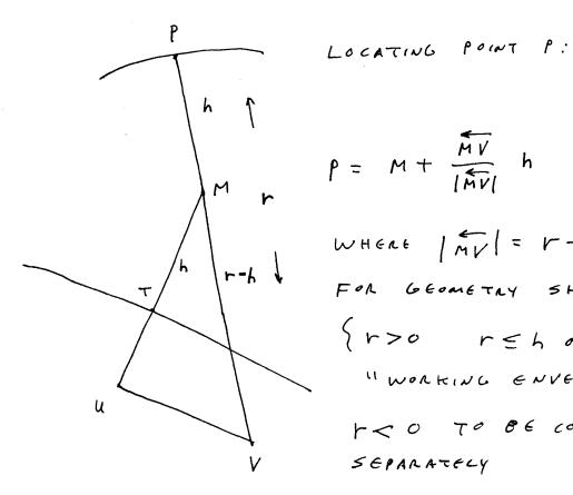
$P = M + \frac{MV}{MV} h$ WHERE INVI = r-h >0 FOR GEOMETRY SHOWN {r>o r=h outside " WORKING ENVELORE " Y CO TO BE CONSIDERED SEPARATELY
