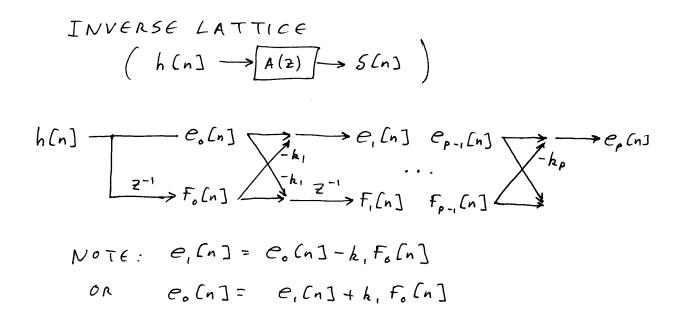
The inverse lattice is simply an expression of the forwardpredictor order update. The forward lattice is the exact same signal flow graph with the directions of the upper path turned around.
