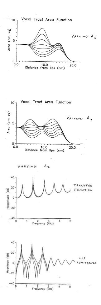
Symmetrical deformation of acoustic tube moves terminal impedance zeroes while leaving formants fixed. Asymmetrical deformation moves formants:
